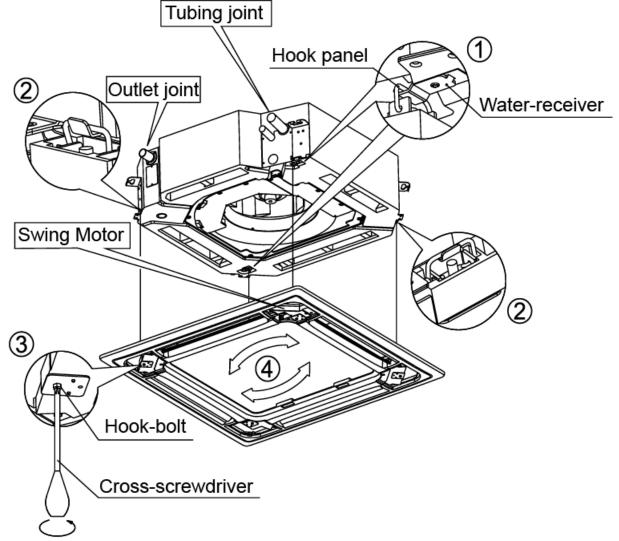
Tighten the screws under the panel hooks till the panel closely stick on the ceiling to avoid condensate water.
