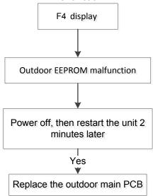
EEPROM: An electrically erasable programmable read-only memory whose contents can be erased and reprogrammed using a pulsed voltage.
