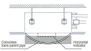
Adjust the position to ensure the gaps between the body and the four sides of ceiling are even. The body's lower part should sink into the ceiling for 10~12 mm. In general, L is half of the screw length of the installation hook.
