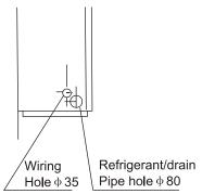
Pipe/wire-hole position on back side
