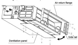
② Stick the attached seal sponge as per the indicating place in the following fig, and then change the mounting positions of air return panel and air return flange.
