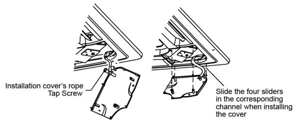
Note: The panel shall be installed after the wiring connected.
