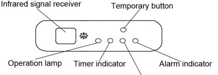
PRE-DEF indicator(cooling and heating type) or fan only indicator(cooling only type)
