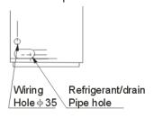
Pipe/wire-hole position on the bottom
