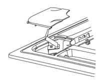
Hang the panel to the hooks on the mainbody. If the panel is with auto-lift grille, please watch the ropes lifing the grille, DO NOT make the ropes enwinded or blocked.
