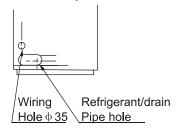
Pipe/wire-hole position on the bottom
