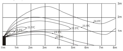
Discharge angle 50° Heating airflow velocity distribution
