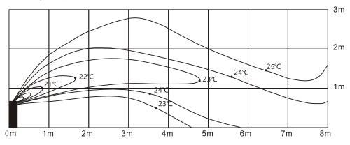
Discharge angle 50° Heating airflow velocity distribution
