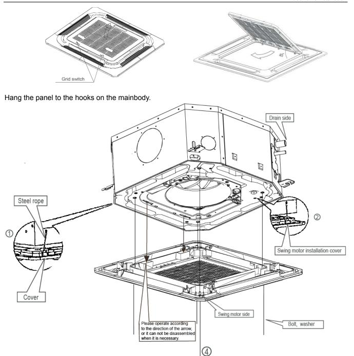
Tighten the screws under the panel hooks till the panel closely stick on the ceiling to avoid condensate water.
