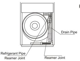
Pipe/wire-hole positions on both sides
